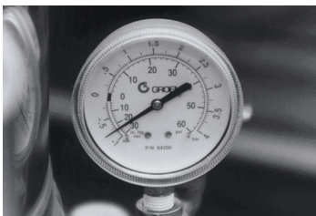
The pressure gauge should show a vacuum of 20 to 30 inches when the kettle is cold.
